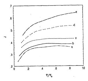
Figure 3: Curves of J vs  $(\psi_r/\psi_b)$ , showing that inversion of the J profile occurs only for configurations highly elongated in the horizontal direction ( $\kappa < 0.5$ ). The curves a, b, c, d and e correspond to  $\kappa = 0.45, \delta = 0.5, q_m = 0.95, \kappa = 0.45, \delta = 0.3, q_m = 0.93, \kappa = 0.45, \delta = 0.0, q_m = 0.82, = 0.60, \delta = 0.3, q_m = 0.99, \kappa = 0.60, \delta = 0.0, q_m = 0.91$ , respectively.
