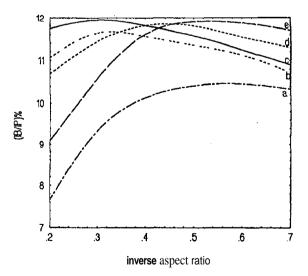
Figure 4: Ratio between the bootstrap and plasma current for the several values of the aspect ratio, for  $\kappa = 1.0, \delta = 0(a), \kappa = 1.0, \delta = 0.2(b), \kappa = 1.5, \delta = 0.5(c), \kappa = 1.5, \delta = 0.2(d)$  and  $\kappa = 1.5, \delta = 0.0(e)$ .
