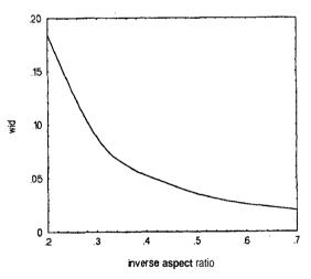
Figure 2: Variation of the banana orbit width normalized to  $\psi_b = \alpha^2 \beta_0 / 4p_1$ , with the inverse aspect ratio, for a proton with energy E = 8.82 Kev.
