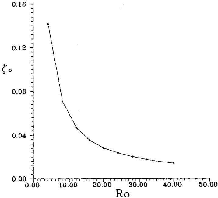
Fig. 3 - Displacement of the magnetic axis  $\zeta_0 = \zeta(r = 0)$ , from the geometric center of the cylinder, versus  $R_0$ , for  $k = 0.5$ ,  $J_0 = 0.5$ ,  $\beta = 0.01$ ,  $a = 4$ .
