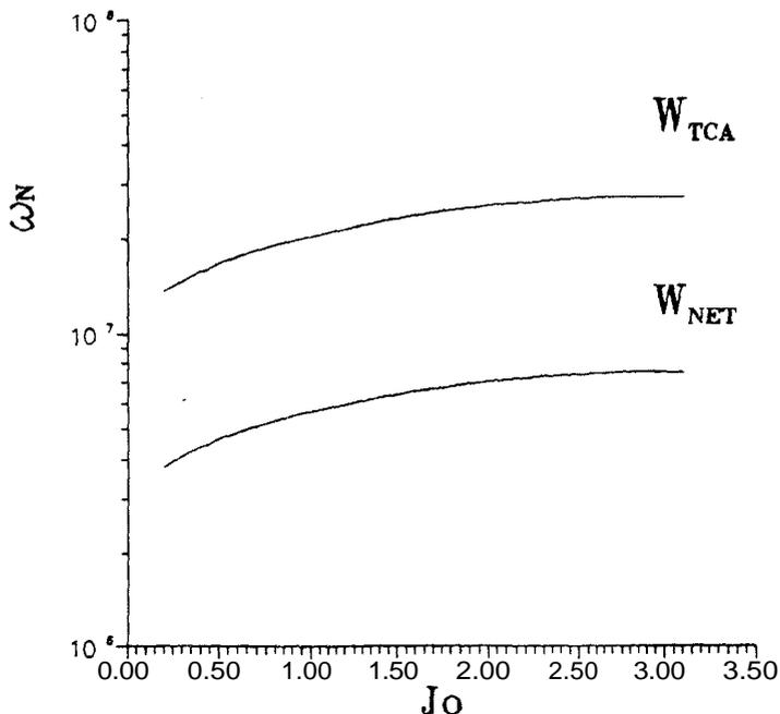
Fig. 4 - Normalized eigenfrequency,  $\omega_N$ , for NET and TCA tokamaks, as function of the normalized current density ( $\sim q_0^{-1}$ ). The following parameters were used:
