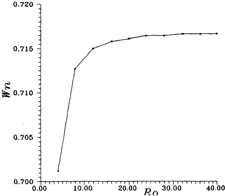
Fig. 2 - Normalized eigenfrequency,  $\omega_N$ , versus  $R_0$  for  $k$  constant ( $k = n/R_0 = 0.5$ ,  $J_0 = 0.5$ ,  $\beta = 0.01$ ,  $\alpha_j = 4$ ). The  $\omega_N$  for the cylindrical plasma column is 0.717.
