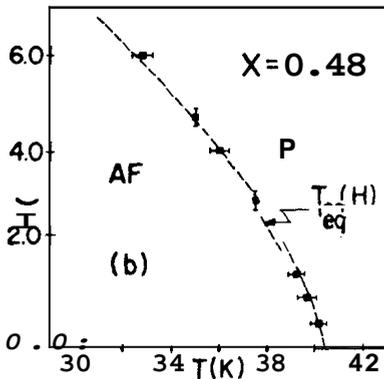
Fig. 2 - Irreversibility phase diagram for  $Fe_{0.48}Zn_{0.52}F_2$ .
