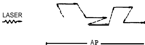
Fig. 1 - Absorption-emission cycles in momentum space for a resonant atom in a laser beam. The full line represents the momentum change after the absorption while the dashed line stands for the change after spontaneous emission. \Delta p is the net momentum transferred to the atom.
