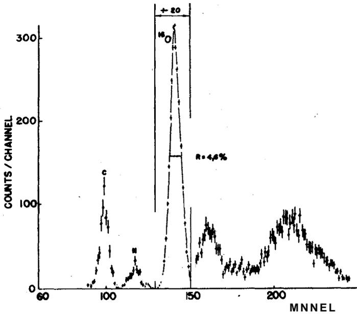
Fig.2 - Spectrum of the AE pulses in coincidence with E pulses, obtained from the reaction  $^{27}\text{Al} + ^{16}\text{O}$ .
