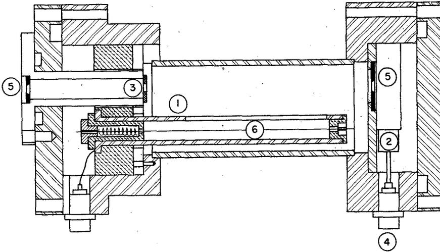
Fig.1 - Vertical cross-section view of the proportional counter: 1. guard-rings; 2. solid state detector; 3. entrance window; 4. microdot connectors; 5. slits; 6. wire.
