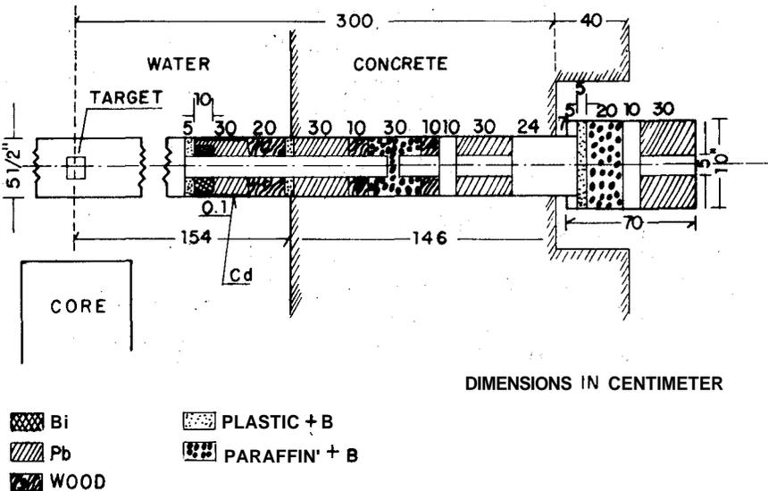
Fig. 2 - Experimental arrangement for  $\gamma$ -radiation production.
