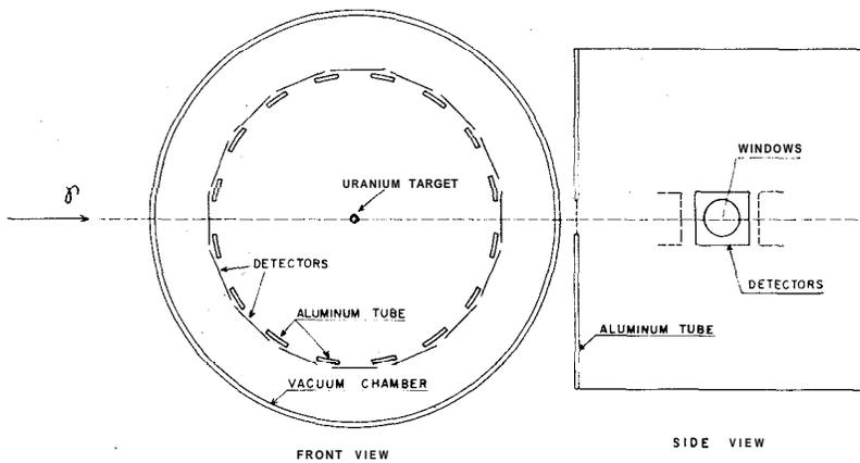
Fig. 3 - Views of the angular distribution experimental arrangement.
