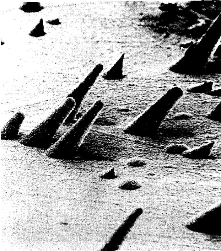
Fig. 7 - A microscopic view of a silicone replica of sulphur ion tracks in a plastic sheet.
