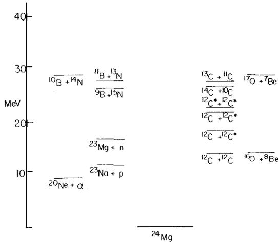
Fig. 5 - The possible breakup modes of  $^{24}\text{Mg}$  are shown up to an excitation energy of 30 MeV.
