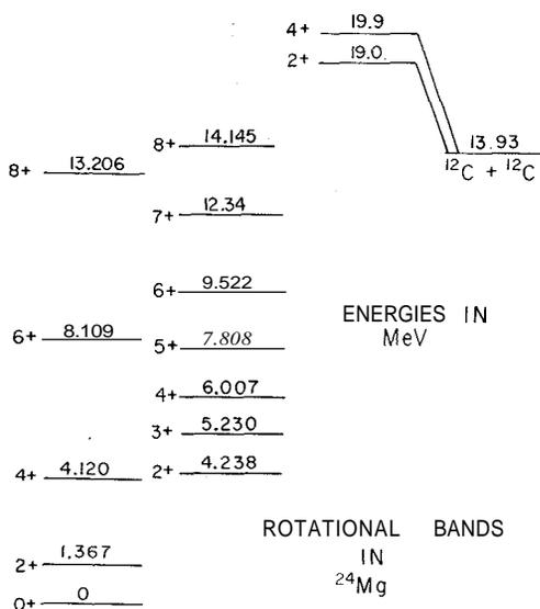
Fig. 3 - Some of the excited states of  ${}^{24}\text{Mg}$ . The two well known rotational bands are shown together with two of the quasmolecular states.
