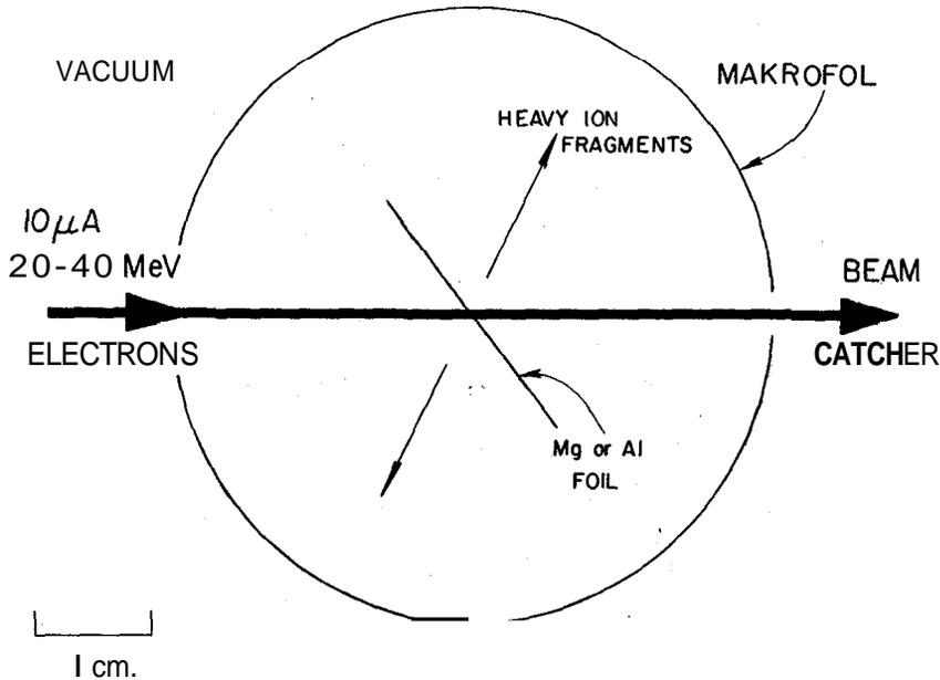
Fig. 9 - The arrangement of electron, target and Makrofol detectors is shown.
