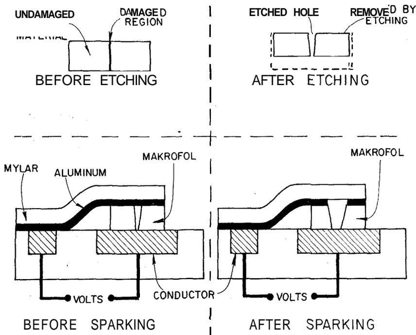
**Fig. 8** - Some details of the sparking technique are illustrated.
