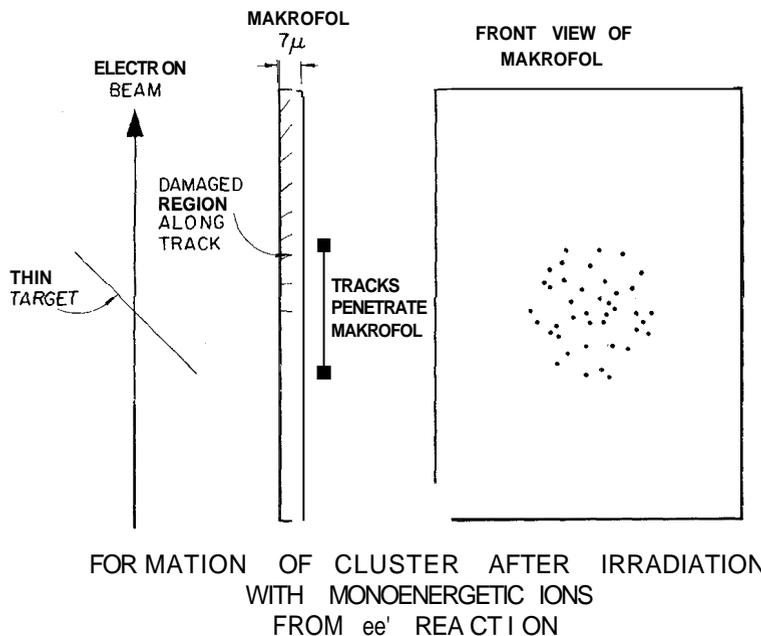
Fig. 2 - The formation of a cluster of holes from monoenergetic heavy ions in a sheet of Makrofol is illustrated.
