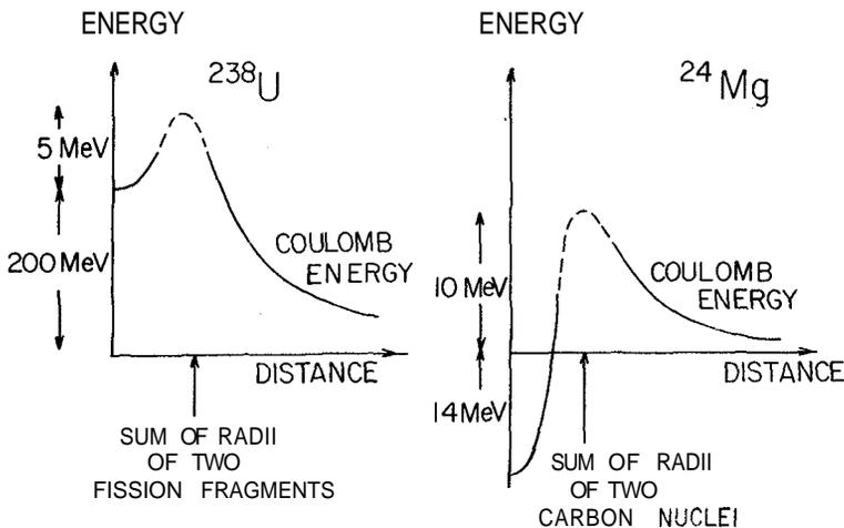
Fig. 1 - Potential energy diagrams to illustrate the differences between the fission of  $^{238}\text{U}$  and  $^{24}\text{Mg}$ . The region shown with dashed lines is not well understood theoretically or experimentally.
