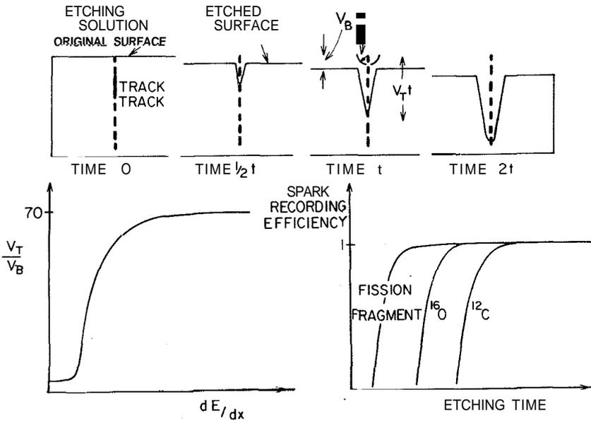
Fig. 6 - The time evolution of the tracks in a plastic film is shown at the top. The ratio of the track etching speed  $V_T$  to the bulk material etching speed  $V_B$  is also shown as a function of the  $dE/dx$  of the heavy ion for cellulose nitrate. A schematic drawing of the spark recording efficiency as a function of etching time for various ions is also shown.
