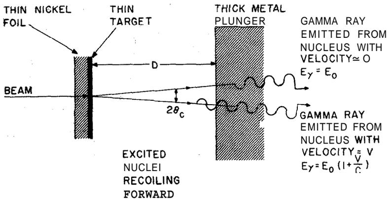
Fig. 8 - Recoil method of measuring lifetimes of excited states (from Ref. 15).
